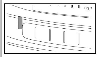
4) Apply tape at right and left edges of part. (Left hand side shown)
