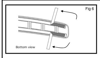
7) Remove part and peel back approximately 30mm of all tape liners.
