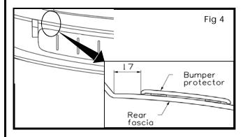
5) Measure the distance from the feature of the rear bumper fascia to the edge of the bumper protector as shown in the figure.
